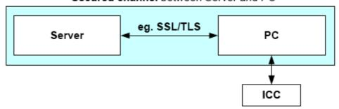
In the above example (taken from EN 14890-2), client/server authentication establishes a secured channel between a remote server and a PC. The ICC will be used as a cryptographic toolbox in order to provide the cryptographic functionality to the PC. If a process needs a certificate from the card that is not provided by OpenPGP (e.g. x.509), then it can be stored in the DO 'Cardholder certificate'.
