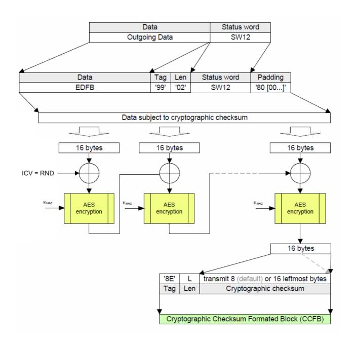
Response APDU computation of cryptographic checksum with AES in CMAC-Mode
