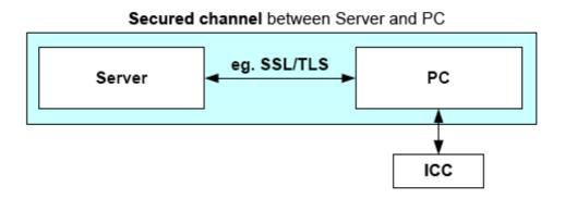
In the above example (taken from EN 419212-5), client/server authentication establishes a secured channel between a remote server and a PC. The ICC will be used as a cryptographic toolbox in order to provide the cryptographic functionality to the PC. If a process needs a certificate from the card that is not provided by OpenPGP (e. g. x.509), then it can be stored in the DO 'Cardholder certificate' (7F21 AUT) as 1st occurrence.
