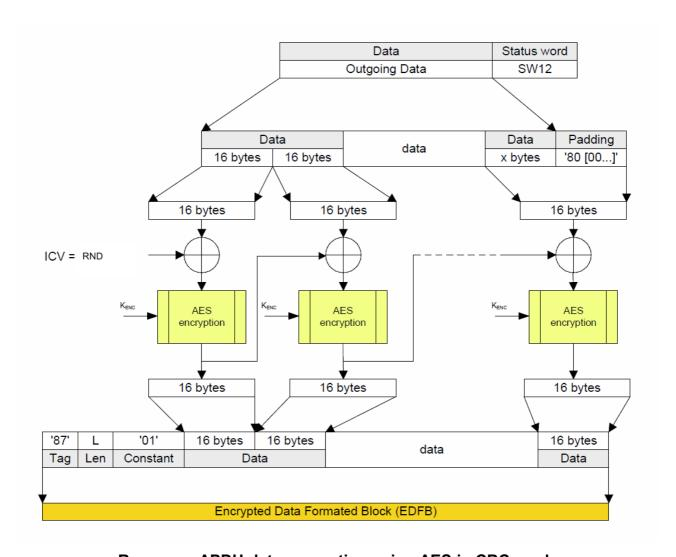
Response APDU data encryption using AES in CBC-mode
