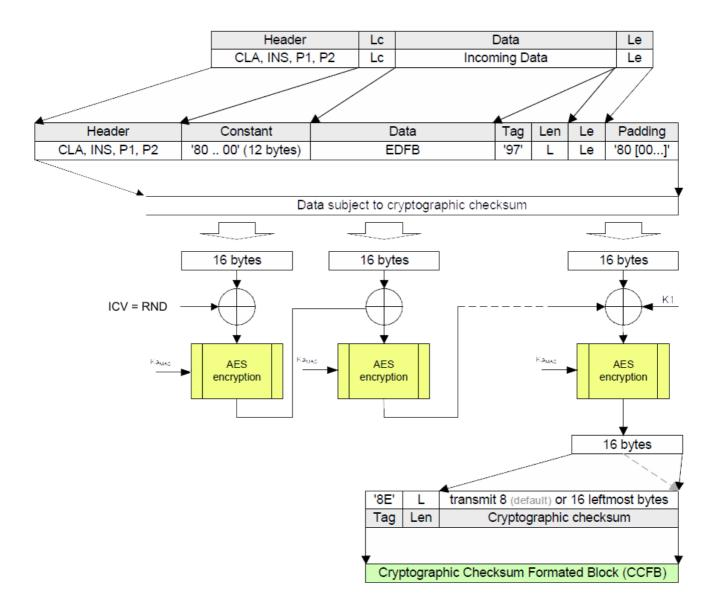
APDU computation of AES cryptographic checksum in CMAC mode
