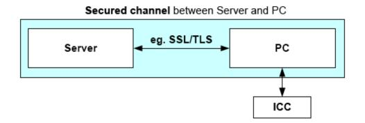
In the above example (taken from EN 419212-5), client/server authentication establishes a secured channel between a remote server and a PC. The ICC will be used as a cryptographic toolbox in order to provide the cryptographic functionality to the PC. If a process needs a certificate from the card that is not provided by OpenPGP (e. g. x.509), then it can be stored in the DO 'Cardholder certificate' (7F21 AUT) as 1st occurrence.
